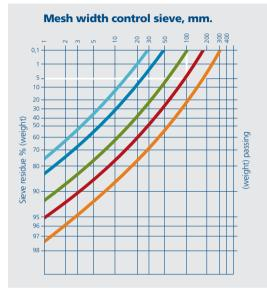
**Example:** To attain a product size distribution with a sieve residue of approximately 5% in a 100 mm control sieve an outlet grate with 125 mm slots is needed.
