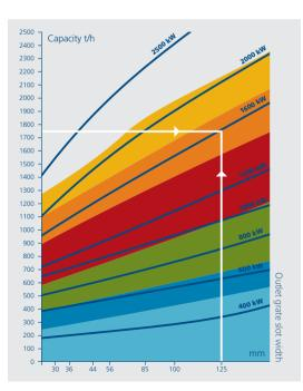
**Example:** An outlet grate with 125 mm slots and a desired capacity of 1750 t/h will result in an EV 250 x 250 with an approximately 1600 kW motor.
